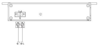
Figure 2-20 Power Connection for EDG-4504
